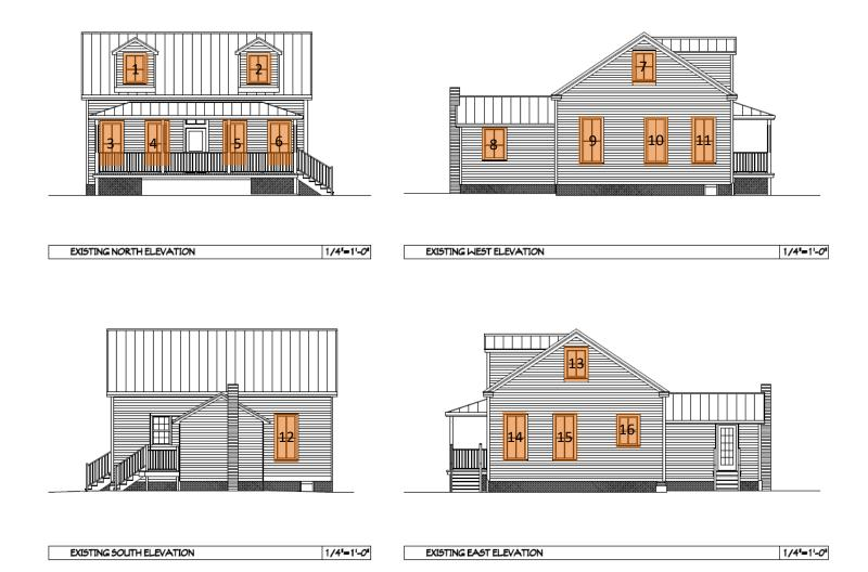
Figure 3 – 16 Additional windows replaced beyond the scope of COA or Building Permit
